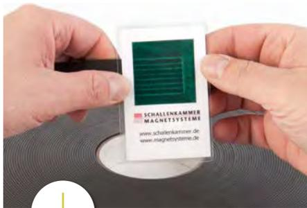
Sensor foil (page 115) visualizes the magnetic field between the magnetic poles.
