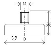
Magnetic system flat, with outer thread,
