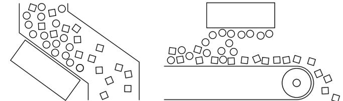
Plate magnets separate ferrous parts.
