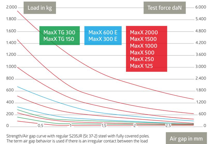
Strength/Air gap curve with regular S235JR (St 37-2) steel with fully covered poles. The term air gap behavior is used if there is an irregular contact between the load and the magnet. This is primarily caused by irregular surface structures or by dirt, color or iron residues on the load's contact surface.
