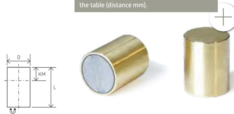
The holding force will be reduced up to 15 percent due to magnetic short circuits when the magnetic system is directly installed in iron. In order to prevent this, certain distances must be observed from the brass housing of the magnetic system to the iron. The distances to the iron shall also be observed when the magnetic system was shortened by the dimension KM. Please see the recommended distances from the table (distance mm).
