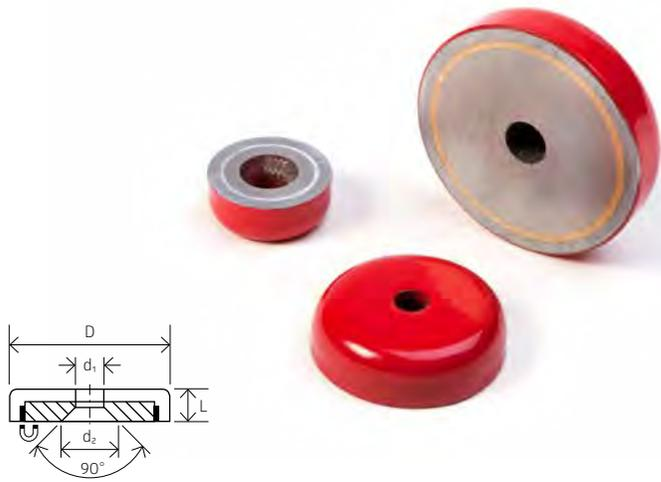
Pot magnet with through borehole and 90° counter bore, magnetic core AlNiCo 500
