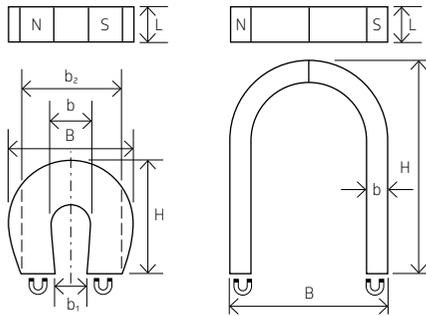
For testing of materials and lifting of small ferrous parts.
