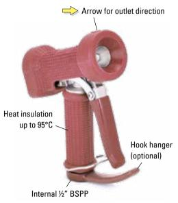
We produce spray guns made of SS 304. Suitable for medium pressure (16 bar), hot water (up to 95°C), 1/2" BSPP internal inlet applied.
